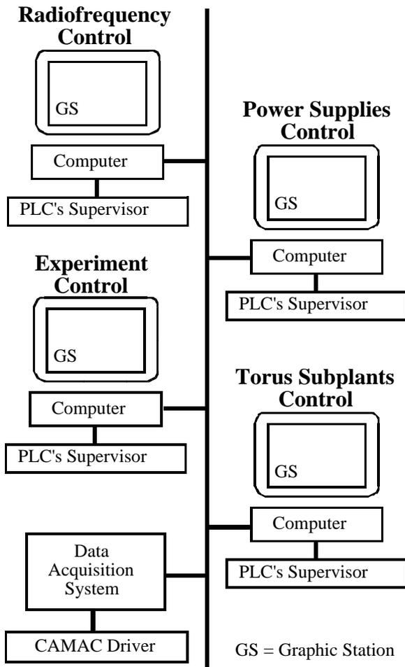
Fig. 1 - FTU control system: block diagram
