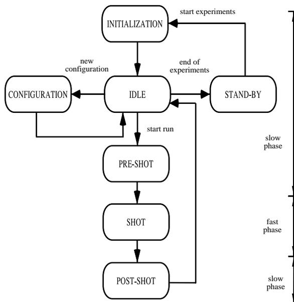
Fig. 1 - Typical Tokamak experiment State Diagram
