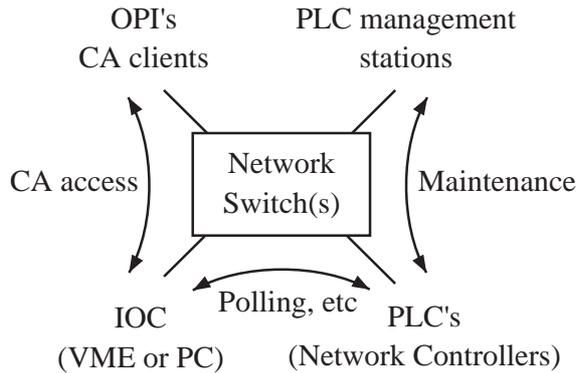
Figure 1: Same network shared among different protocols. Message packets for different purposes are ordered by network switches and do not interfere with each other.
