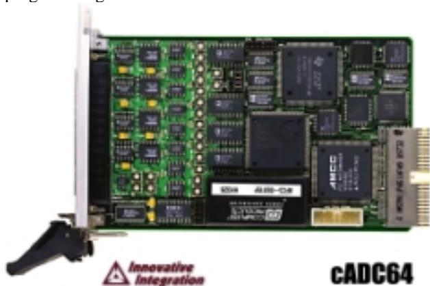
Figure3: The CompactPCI I/O card, from Innovative Integration, with a TMS320C32 DSP on board.
