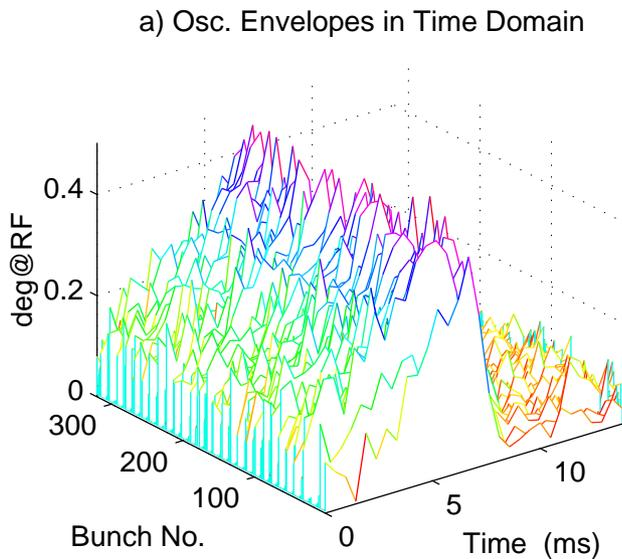
Figure 3: Envelopes of bunch oscillation show growing motion followed by damping
