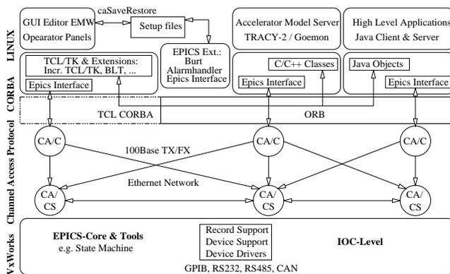
Figure 1: Layout of the Control Software Layers.
