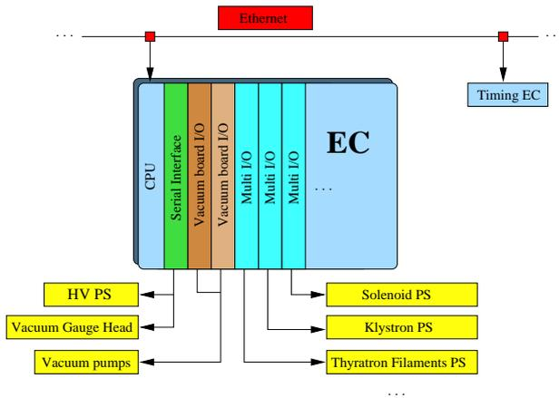
Figure 2: Equipment Controller layout
