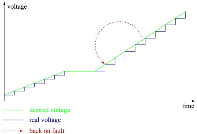
Figure 3: High Voltage ramp
