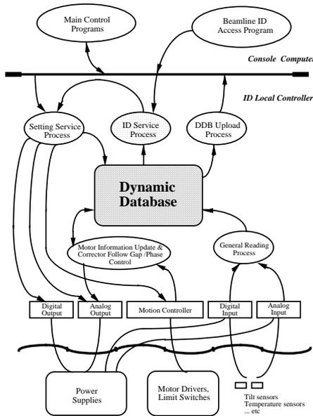
Figure 1: Structure of the EPU5.6 control software.
