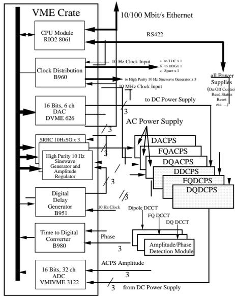
Figure 4. 1.5 GeV booster power supply control interface
