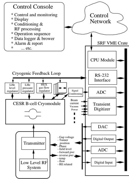
Figure 5. Superconductivity RF system – control environments
