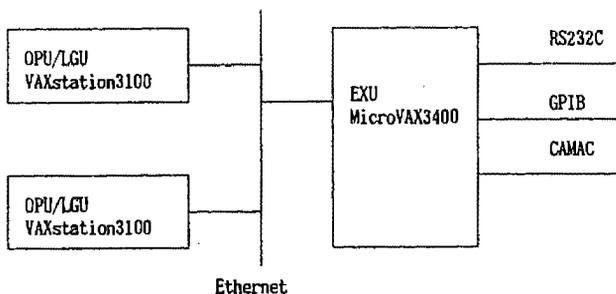
Fig.1 The new computer control system of TARN2
