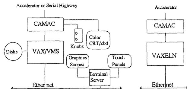
Figure 1. LAMPF Operator Interface and Front End Computers
