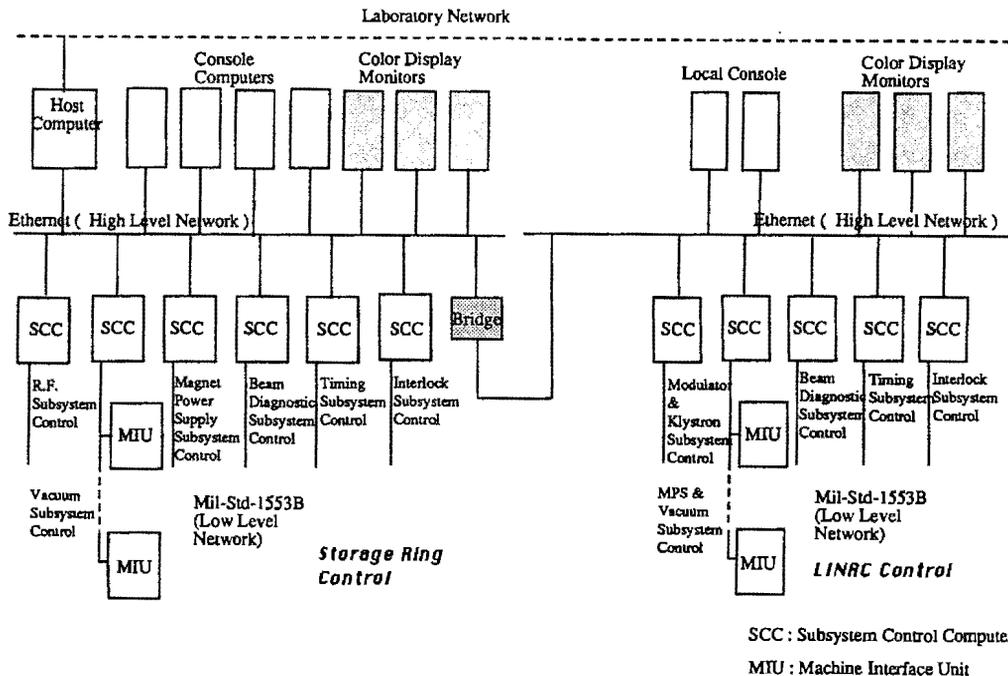
Figure 1. PLS Control System Architecture
