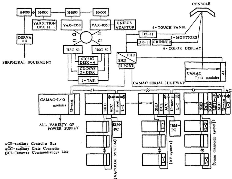
Fig.1 The block diagram of HIRFL control system
