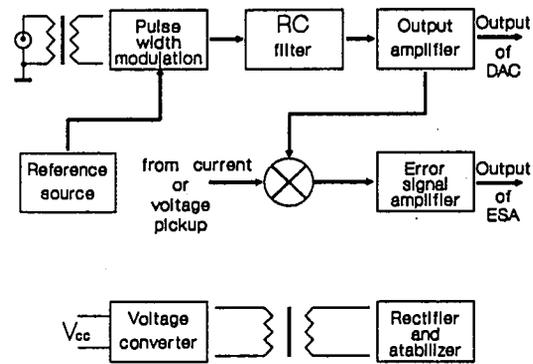
Fig.1. The analog section of PWM-DAC.
