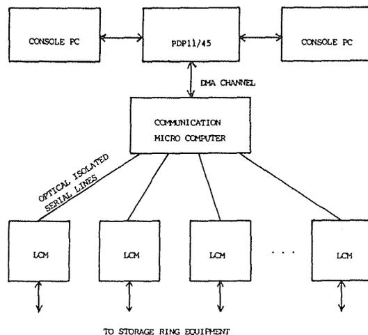
FIG. 1 BLOCK DIAGRAM OF HESYRL RING CONTROL SYSTEM
