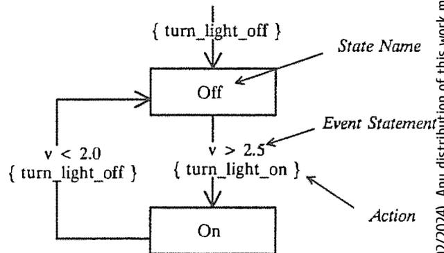
Figure 1. Example of a State Transition Diagram.
