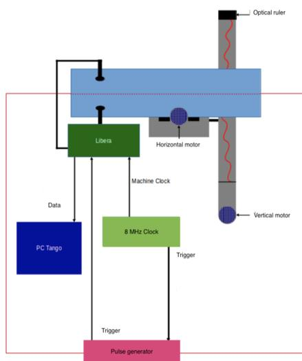
Figure 3: Measurement setup: a pulse generator is used to send pulses on the stretched wire and trigger signals to the machine clock (8 MHz generator) and to the libera. The libera reads the signal on the four electrodes of each of the three BPMs. The data recorded by the libera are read by a PC using Tango.
