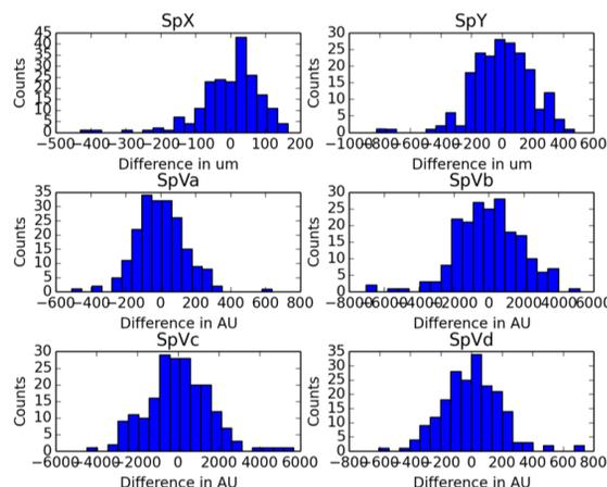
Figure 7: Difference between the position calculated by drawing a straight line between the two outer BPMs and the central one.
