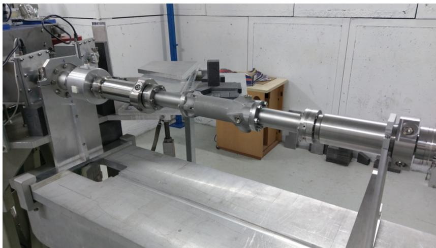
Figure 5: The BPM triplet installed on PHIL. The beam is coming from the left to the right. On the picture one can see (from left to red), first an ICT then one of the conventional BPM, the 3D-printed BPM and the other conventional BPM. There is no magnetic element between the BPMs.
