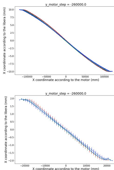
Figure 4: Position measured by the three BPMs (after calculation by the Libera). The horizontal axis shows the estimated position according to the number of steps sent to the motor and the vertical axis shows the measured position. To make the figure easier to read an offset has been applied to the value read by the BPMs so that of the three BPM are reading 0 when the motor is at position 0. The red dots correspond to the 3D-printed BPM and the blue and green dots to the conventional BPM.
