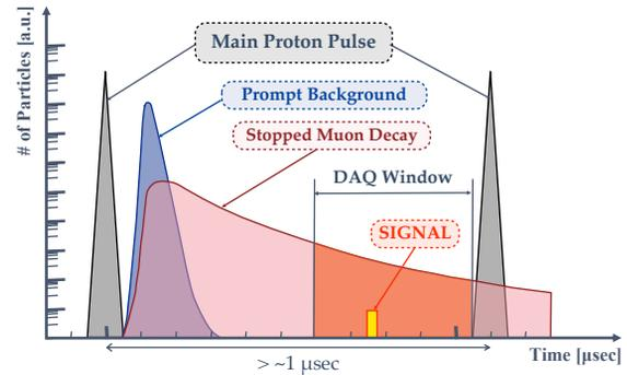
Figure 1: Time structure of the proton beam, background events and DAQ window for the COMET Experiment.
