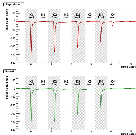
Figure 6: Quick test with different kicker timings; (*top*) Reproduced K4-rear Mystery with 600 nsec kicker shift, (*bottom*) Suppressed K4 leakage with 750 nsec kicker shift.
