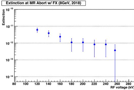
Figure 4: Obtained extinction factor at Abort with FX beam as a function of applied RF voltages.
