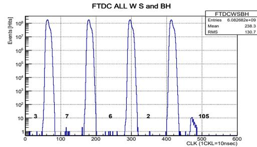
Figure 5: Obtained timing spectra of delivered pions; (top) Number of hit entries of hodoscope as a function of relative timing with respect to the injection-batches timing, (bottom) Timing spectra with lower RF voltage of 30 kV.
