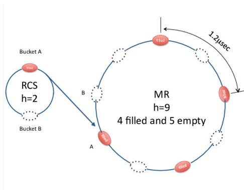
Figure 2: Dedicated beam transfer diagram from RCS to MR to COMET to make the long enough bunch intervals.
