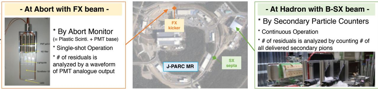
Figure 3: Two measurement schemes at the Abort with FX beam and at the Hadron with Bunched-SX beam.
