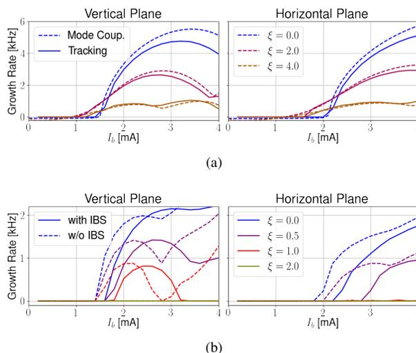
Figure 4: Transverse single-bunch instabilities for the first phase of operation of the Sirius storage ring, a) without b) with the effects of IBS and potential-well distortion.
