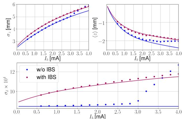
Figure 2: Main parameters of the beam obtained from tracking (dots) as a function of the current for the simulations with and without the effects of IBS. The values shown here are averages over all the  $3 \times 10^4$  turns of the simulation. The solid lines are the results obtained from the solution of the Haissinski equation.
