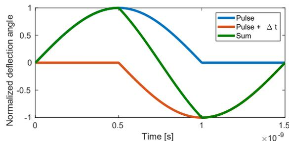
Figure 5: Combining two stripline pulse to reduce the fall time
