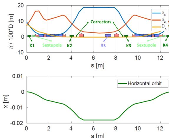
Figure 1: ESRF-EBS injection cells
