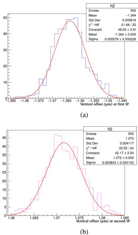
Figure 6: Vertical offset of the weak beam in the presence of beam-beam elements (a) at the first IP and (b) at the second IP.
