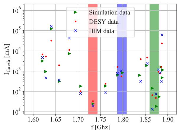
Figure 6: Simulation of threshold current values for different data sets. Red: All values from simulated data, blue: Q and f values from vertical cold test measurements at DESY and green: Q and f values measured in the cryomodule tuned to 1.3 GHz.
