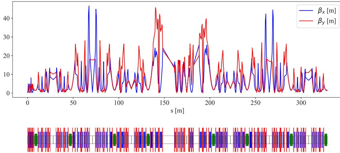
Figure 3: Horizontal and vertical beta functions along the beamline for a start to end ERL configuration of MESA simulated in ELEGANT [5]. The layout below the graph depicts the optical elements. Dipole magnets are blue, quadrupole magnets are red and accelerating/decelerating cavities are green.
