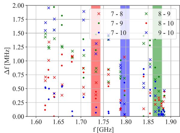
Figure 5: Comparison of absolute frequency deviation between cavity HOMs as measured at HIM.
