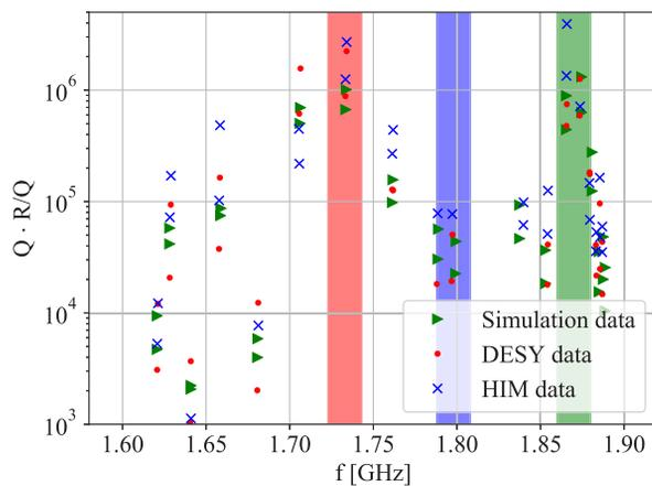
Figure 4: Comparison of measured and simulated  $Q \cdot R/Q$  values shown for cavity 7. The cavities are numbered from 7 to 10 with cavity 7 and 8 in one module and 9 and 10 in the other one.
