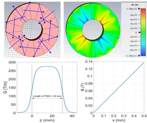
Figure 5: CST simulations of PMQ. Top figure shows the direction of magnetization and the corresponding field density plot. The bottom figure gives the maximum achievable gradient and field amplitude
