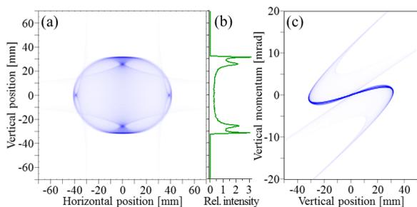
Figure 3: Tracking simulation result of the 10-MeV proton beam focused using two octupole magnets. The beam-line parameters are the same as those in Fig. 2(b). (a) Relative intensity distribution of the beam cross-section. (b) One-dimensional relative intensity distribution along the vertical axis in (a). (c) Phase-space distribution in the vertical direction.
