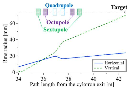
Figure 1: Schematic layout of magnets and transverse beam envelope calculation near the hollow-beam formation target. The root-mean-square (rms) emittance assumed is  $2\pi$  mm·mrad in the horizontal direction and  $1\pi$  mm·mrad in the vertical direction. Two sets of sextupole and octupole magnets have been installed beside the final quadrupole doublet.
