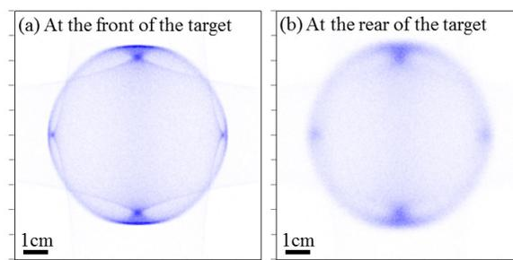
Figure 4: Cross-sectional profiles of the hollow beam at the front and rear of the target. The on-target shape of the beam has been transformed from an ellipse (Fig. 3) into a circle by adjusting the beam optics. For simplicity, particles in the hollow beam are kicked randomly at the front of the target with an average angle of 8 mrad, which corresponds to the multiple-scattering angle of a 392 MeV proton beam in a 20-cm-long graphite (2.3 g/cm<sup>3</sup>).
