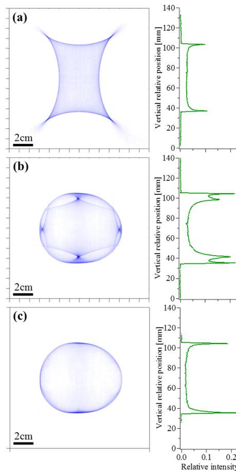
Figure 2: Spatial intensity distributions of the 10-MeV proton beam focused with one or two octupole magnets. The strengths ( $K_{OCT1}$ ,  $K_{OCT2}$ ) of the two octupole magnets are (a) ( $0 \text{ m}^{-4}$ ,  $3100 \text{ m}^{-4}$ ), (b) and (c) ( $-10500 \text{ m}^{-4}$ ,  $3100 \text{ m}^{-4}$ ). In (c), the beam tail has been collimated. The left and right panels are the cross-sectional and vertical axial distributions of the beams, respectively.
