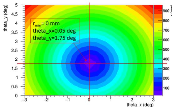
Figure 6: The relationship between steering angles and beam spot deviation.
