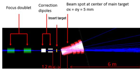
Figure 5: Proton beam steering layout for EMuS.
