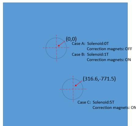
Figure 7: The two beam spots at the beam dump with proton beam steering scheme.
