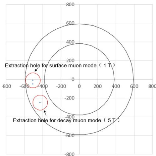
Figure 9: Extraction channels of the spent protons at the extraction plane.
