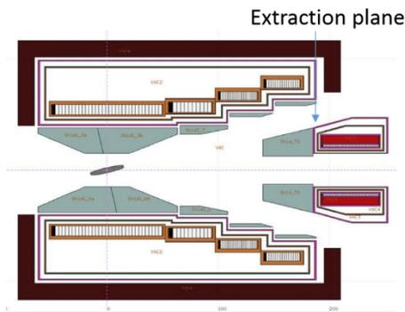
Figure 8: Layout of solenoids structure and proton extraction space.
