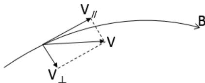
Figure 3: The protons motion decomposition in the solenoid field.
