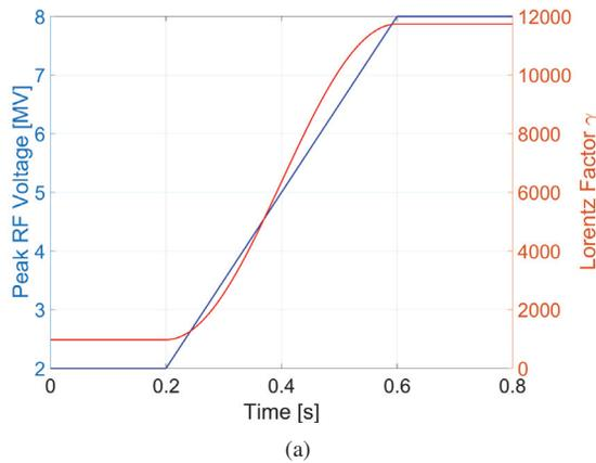
Figure 1: Ramping curves of the peak RF voltage (in blue color) and the corresponding Lorentz factor (in red color)  $\gamma$ .
