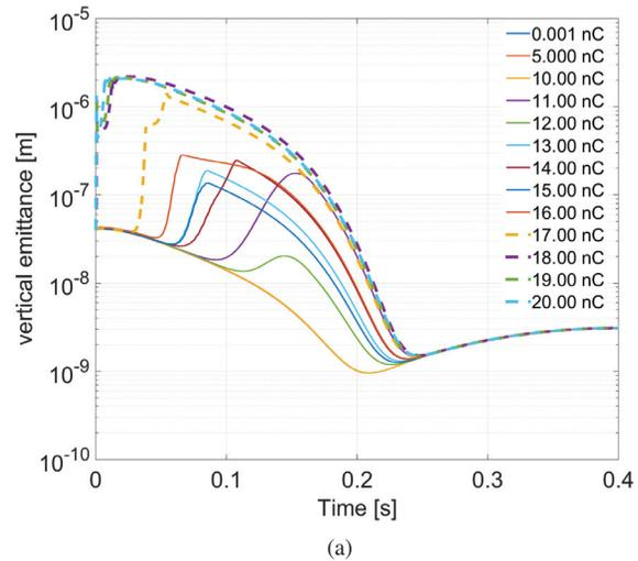
Figure 5: Vertical emittance vs. time under the condition that the bunch energy ramps immediately after injected at 500 MeV, corresponding to the green curve in Figure 4. The dashed curves represent the situations with particle loss, while the solid curves are the cases without particle loss.
