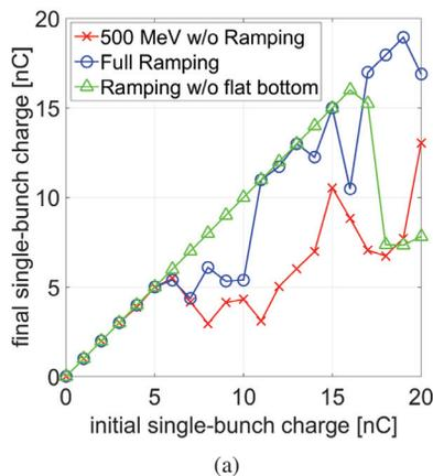
Figure 4: Comparison of the single-bunch charge threshold under the conditions with and without the consideration of energy ramping.
