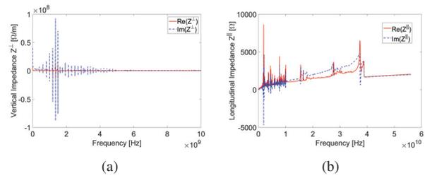
Figure 2: Vertical (a) and longitudinal (b) impedance used in the tracking simulations.
