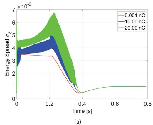
Figure 3: Variation of energy spread in the ramping process.
