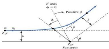
Figure 4: Schematic figure of general Rutherford scattering. In this figure, the incoming particles are positively charged whereas they are electrons in this paper. But,  $\theta$  has the same magnitude just with negative sign.
