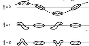
Figure 1: This figure shows longitudinal modes of head-tail instability.  $l = 0$  is the dipole mode and  $l = 1, 2$  are next higher modes.
