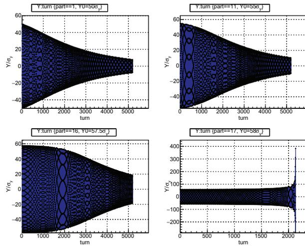
Figure 4: Time evolution of vertical oscillations for particles with initial vertical coordinate  $y = \{50; 55; 57.5; 58\} \times \sigma_y$ , horizontal coordinates are zero, longitudinal are adjusted for synchronous point.
