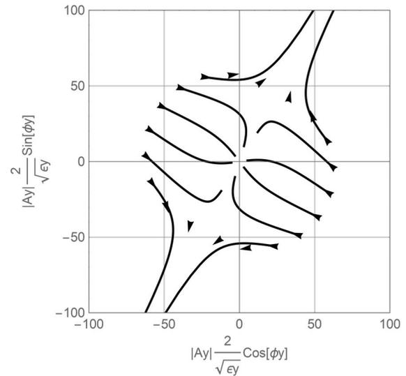
Figure 5: Evolution of the average particle trajectories, solution of equations (4) and (5) with the same initial amplitude and different initial phases. Initial amplitude corresponds to  $y_0(\varphi_y = 0) = 58\sigma_y$ .
