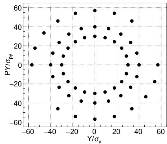
Figure 6: Vertical dynamic aperture from tracking in  $Y, PY$  plane.
