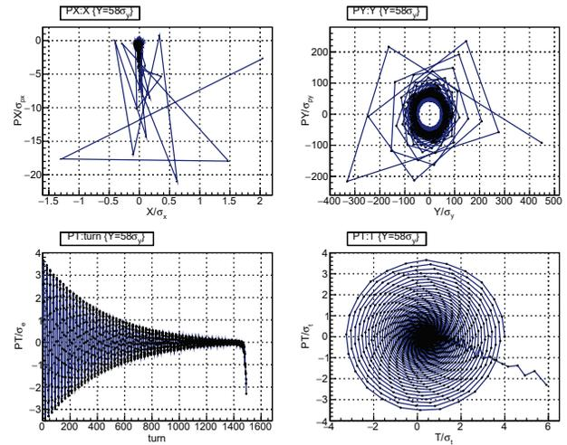
Figure 2: Phase and time trajectories of the first unstable particle with initial conditions  $\{x = 0, y = 58\sigma_y, p_x = 0, p_y = 0, \sigma = 0, p_\sigma = 0\}$ .
