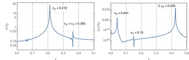
Figure 3: Spectrum of vertical (left) and longitudinal (right) motion from tracking corresponding to initial condition  $y = 58\sigma_y$ , and adjusted longitudinal initial conditions.
