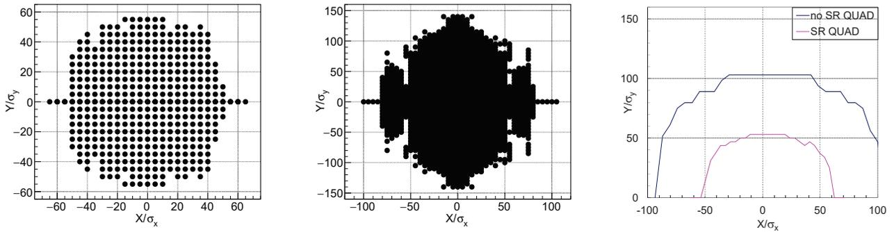
Figure 1: Dynamic aperture: left — tracking by MADX PTC with synchrotron radiation from all magnetic elements, center — tracking by MADX PTC without synchrotron radiation from all magnetic elements, right — tracking by homemade software with synchrotron radiation from quadrupoles (blue) and without (magenta).
