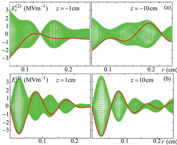
Figure 3: CR field ( $E_r$  component) at the third CR mode ( $\approx 386$  GHz), in the coaxial area (a) and in wide vacuum waveguide (b). Parameters:  $b = 0.064$  cm,  $a = 0.25$  cm,  $\varepsilon = 3.8$ ,  $q = 1$  nC,  $\beta = 0.9999$ ,  $\sigma = 0.012$  cm,  $L = 6.45$   $\sigma$ .
