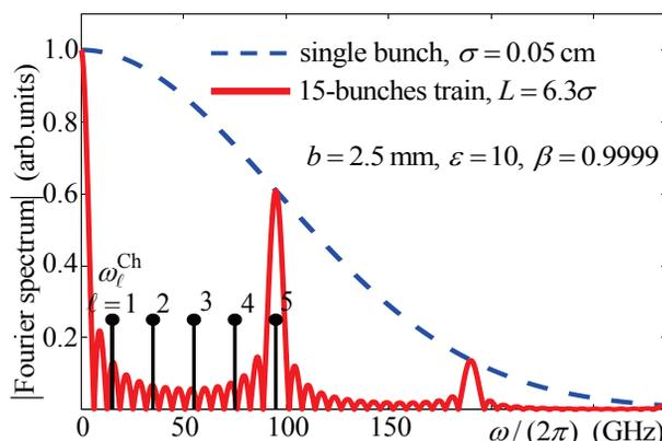
Figure 2: Typical Fourier spectrum of a single Gaussian bunch and that of a 15 bunches train with  $L > 2\sigma$  spacing, black markers show CR frequencies.
