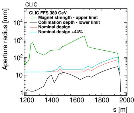
Figure 5: Extended apertures distribution in the Final Focus System at 380 GeV.
