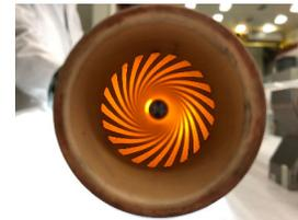
Figure 7: Prototype of the spiral beam screen (photograph).
