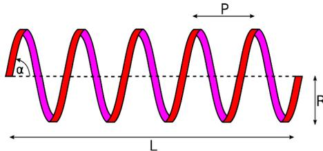
Figure 3: Schematic of a single spiral conductor.
