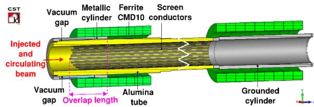
Figure 1: Schematic of the conventional beam screen.
