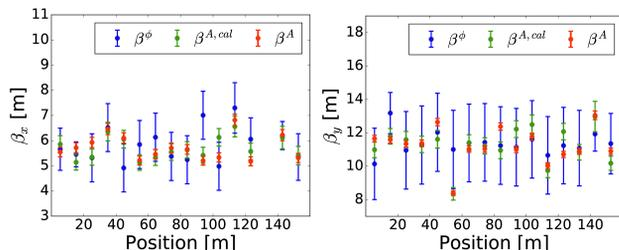
Figure 2: Measured  $\beta^\phi$ ,  $\beta^A$  and  $\beta^{A,cal}$  functions for the Q4Q4 optics as a function of position: horizontal (left), vertical (right). BPMs connected to the radial feedback have not been calibrated due to the noise introduced in the turn-by-turn measurement.
