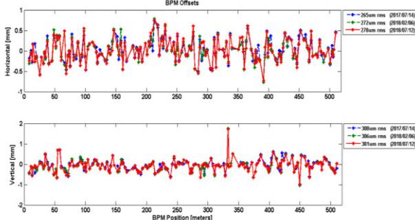
Figure 12: Results of BBA measurement.
