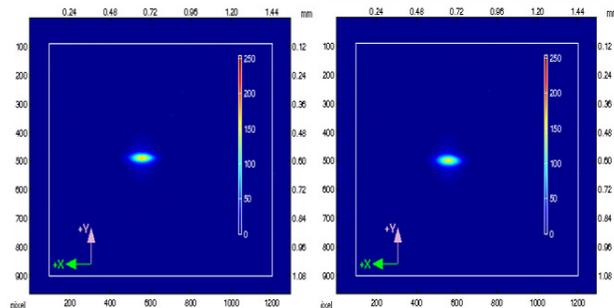
Figure 11: Beam profile before coupling correction (left) and after correction (right).
