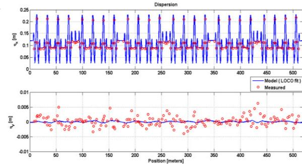
Figure 5: Dispersion function measurement after optics correction (red circle: measured data, blue line: LOCO result).
