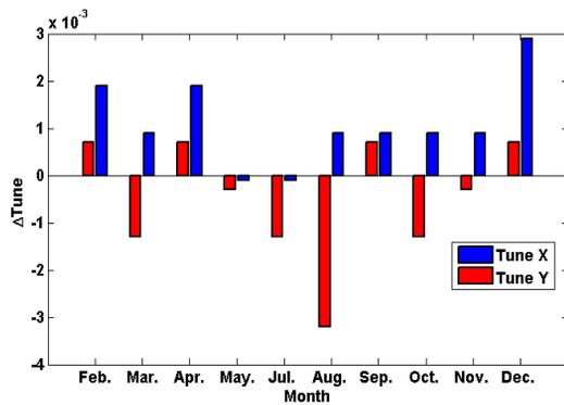
Figure 10: Betatron tune differences after optics correction.
