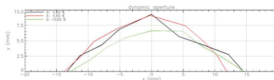
Figure 4: Dynamic aperture for the sextupole scheme used for injection. Since we do not constrain the bypass sextupoles to maximize the nonlinear acceptance, their strengths may be reduced and the dynamic aperture improved.
