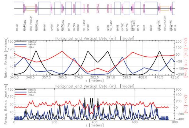
Figure 1: Layout of the OSC bypass, as well as the linear optics within the bypass and in the full ring.
