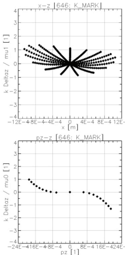
Figure 2: The nonlinear transverse and energy acceptance. No cooling will occur for particles with  $|k\Delta L/\mu_1| > 1$  due to a transverse offset or  $|k\Delta L/\mu_0| > 1$  due to an energy deviation. Three standard deviations in the beam size and energy spread are plotted.
