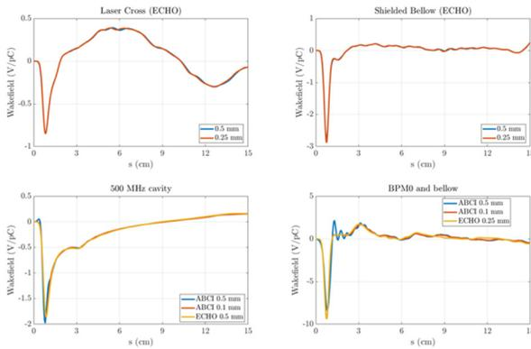
Figure 4. wakefields (around bunching cavities) simulated in ABCI and ECHO have decent agreement.
