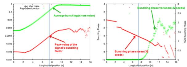
Figure 11. GENESIS simulated evolution of bunching factor of an imprint indicates we have plenty of gain for cooling (left). We operate our FEL in linear regime where phase variation due to shot noise stays low (right).
