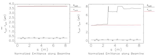
Figure 9. beam emittance can be blown up when the energy spread is large (~1%, right). The emittance growth in dogleg is minimal while energy spread is reasonably low (~0.1%, left).
