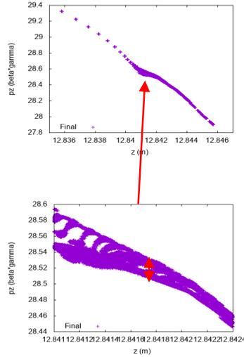
Figure 5. longitudinal phase space at the end of linac shows the beam has a core with peak current  $> 100$  A and slice energy spread  $< 2e-4$  with correlated energy chirp  $\sim 2e-4$ . The core consists of  $\sim 80\%$  of the total charge of 1 nC.
