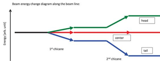
Figure 4: Using two chicanes with opposite bending directions (thus opposite D and D'), it is possible to compensate the emittance growth by cancelling the transverse effects induced by CSR wakes. Change in energy in second chicane is stronger due to stronger wakes – shorter bunch length, thus the bending strength should be smaller. Phase advance between two chicanes can be tuned to realign different longitudinal slices – reduce the overall projected emittance.
