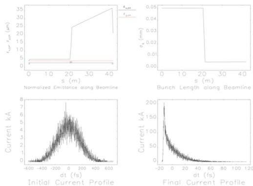
Figure 2: A conventional C-type chicane shows in order to compress the beam to 200 kA peak current, the emittance grows to 5 times after the chicane.
