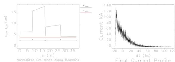
Figure 5: Emittance growth due to CSR effect is largely cancelled in 2<sup>nd</sup> chicane of a zigzag chicane with optics tuning to align slices in between.
