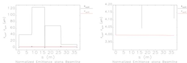
Figure 8: Emittance growth for a 30-fold bunch compressor is < 3% with initial momentum chirp of 1600.
