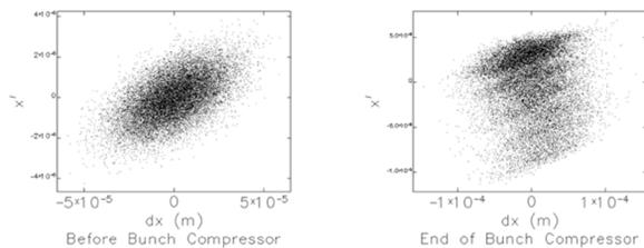
Figure 3: Phase-space distribution before (left) and after (right) the bunch compressor. The longitudinal energy variation induced by CSR wakes is coupled to the coordinate and angular displacements through R16 and R26 induced in the chicane. This results in smearing of the transverse phase space.
