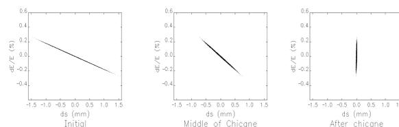
Figure 1: The beam, with an initial energy chirp, rotates and compresses in a C-type chicane.
