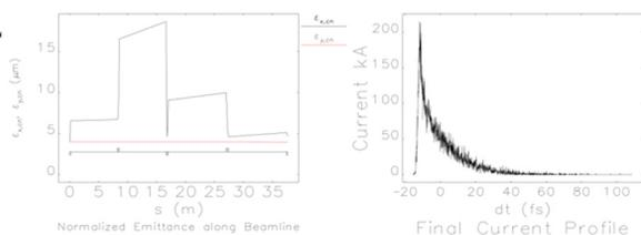
Figure 6: Further increase the compression strength results in a beam with peak current > 200 kA and emittance ~ 4.66 um, 16.5% growth before compression.
