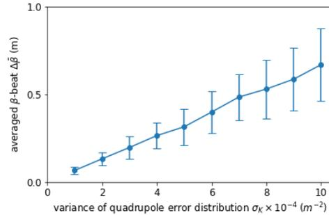
Figure 1: Statistic illustration of the horizontal  $\beta$ -beat due to the random quadrupole errors. This linear correlation with gradually increasing variance are calculated with the NSLS-II ring lattice model in advance. Once an averaged  $\beta$ -beat is measured, its corresponding variance of quadrupole error distribution can be used as the prior probability to prevent overfitting
