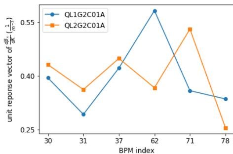
Figure 2: The unit  $\beta_x$  responses vectors of quadrupole 10 and 11 seen at 6 selected BPMs. They are near-orthogonal because their correlation is as low as 0.0612.
