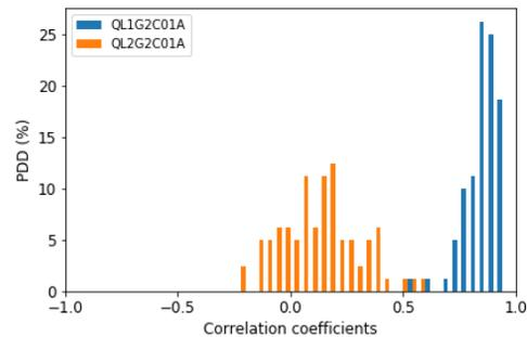
Figure 3: The probability density distribution (PDD) of the correlation coefficients between 800 measured  $\beta_x$  distortion and two unit vectors  $\mathbf{v}_{10,11}$ . The independently and repeatedly measured  $\beta$ -beats are highly correlated with quadrupole 10's pattern, rather than its neighbor. Based on that we can conclude that the actual error source is more likely from the quadrupole 10 (QL1G2C01A) instead of quadrupole 11 (QL2G2C01A).
