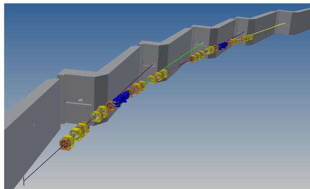
Figure 2: Fitting the existing beam-line layouts and the ratchet wall extraction ports with the new TBA lattice. Two longitudinal gradient bends and two reverse bends are not shown in this plot.
