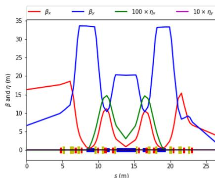
Figure 1: Linear optics and magnetic lattice layout for one TBA cell. A supercell is composed of two such symmetrical cells. This layout provides the same number of alternating high- and low- $\beta$  straights as the existing NSLS-II ring.
