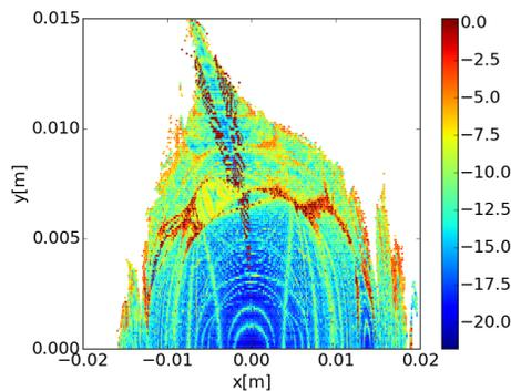
Figure 5: On-momentum dynamic aperture observed at the high  $\beta$  straight section. The color represents the tune diffusion rate in turn-by-turn tracking.
