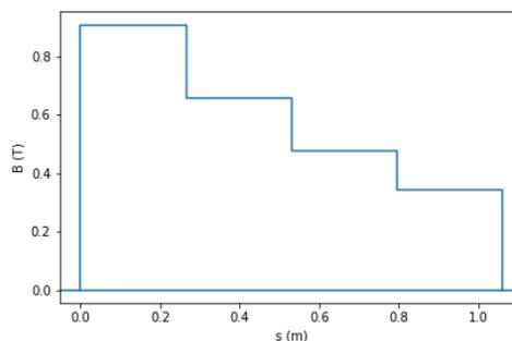
Figure 3: Profile of the vertical magnetic field strength along the upstream longitudinal coordinates for the gradient dipole. The magnet is simply modelled as a hard-edge dipole array. The downstream one is symmetrically mirrored to it.
