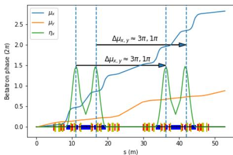
Figure 4: Interleaved betatron phase pattern within a supercell. Four dispersion bumps, inside of which the chromatic sextupoles are located, have a cross-cell interleaved phase cancellation scheme for both the horizontal and vertical planes.
