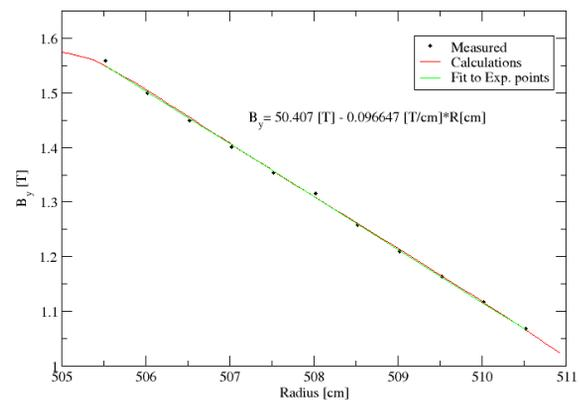
Figure 9: Measured  $B_y$  component (black dots) along the radius at the median plane  $y=0$  (red line in Fig. 7). The red curve on the plot is the calculated  $B_y$  component of the magnetic field as calculated by the OPERA computer code. The green line is a straight line fit to the measured values.
