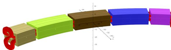
Figure 2: Perspective view of the iRCMS cell showing all five magnets of the cell and the coil.
