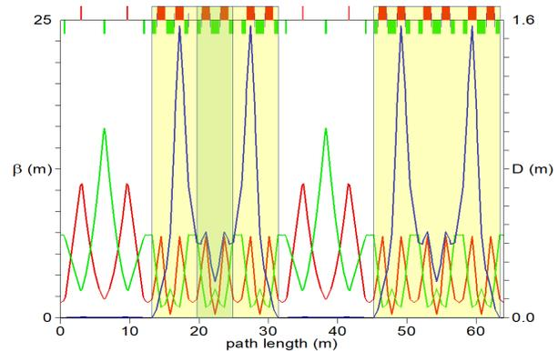
Figure 5: Plot of the  $\beta_{x,y}$  and  $\eta_{x,y}$  functions of the iRCMS ring. The yellow highlighted areas are the  $180^\circ$  arcs of the iRCMS and the green highlighted area is the middle cell of one of the  $180^\circ$  arcs.
