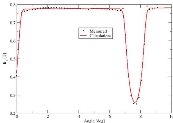
Figure 8: Measured  $B_y$  component of the field (black dots) along the arc  $R=508.022$  cm at the median plane  $y=0$ . The red curve is the  $B_y$  component of the magnetic field as calculated by the OPERA computer code.
