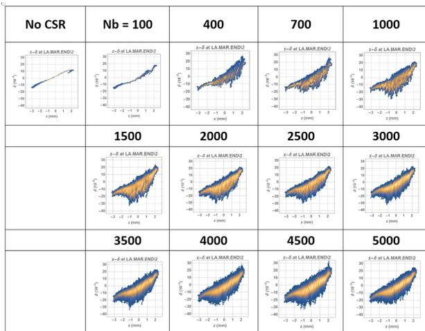
Figure 3: Fig. 1: The results of CSR tracking of a  $Q = 25$  pC bunch with the CBETA 1-pass lattice and varying  $N_b$ .
