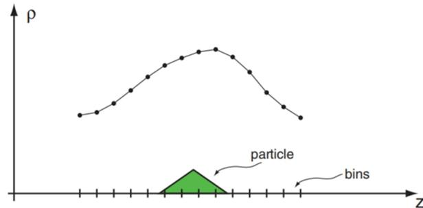
Figure 2: Bmad implementation of CSR. The bunch is divided into a number of bins to allow numerical calculation of the CSR kick.
