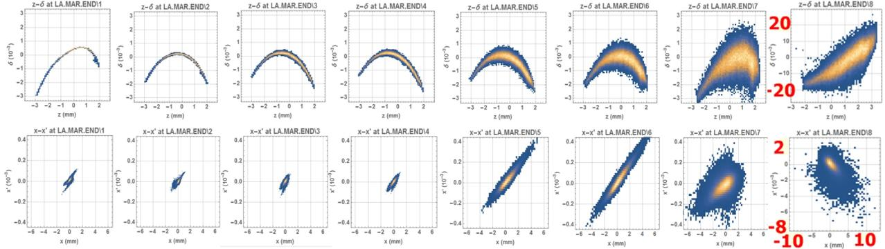
Figure 6: The  $x - x'$  and  $z - \delta$  distributions after each of the 8 LINAC passes for CBETA 4-pass with  $Q = 1$  pC.
