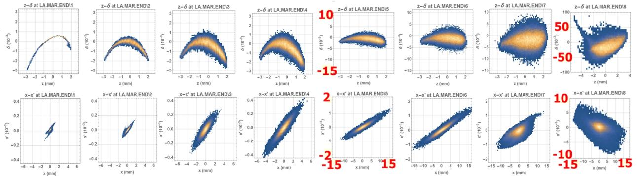
Figure 7: The  $x - x'$  and  $z - \delta$  distributions after each of the 8 LINAC passes for CBETA 4-pass with  $Q = 5$  pC.
