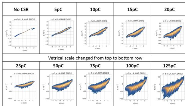
Figure 4: The  $z - \delta$  distribution after each of the 8 LINAC passes for CBETA 1-pass with various  $Q$ .
