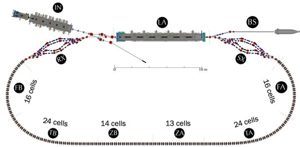
Figure 1: Layout of the CBETA accelerator. The section labeled (LA) is the accelerating LINAC. The sections labeled (SX) and (RX) are the splitters which control the beam optics and time of flights of each recirculation pass. The sections labeled (FA), (TA), (ZA), (ZB), (TB), and (FB) form the FFA beamline which can accommodate four recirculating orbits with an energy range from 42 MeV to 150 MeV.
