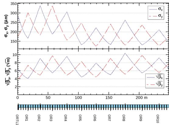
Figure 3: Optics of 1.54-6 GeV linac.
