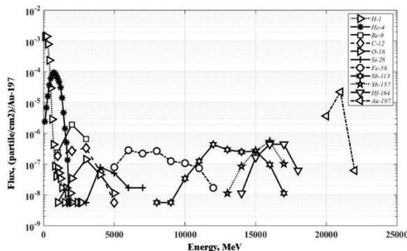
Figure 8: Spectrum of secondary particles at the ion energy degradation in the chip capsule.
