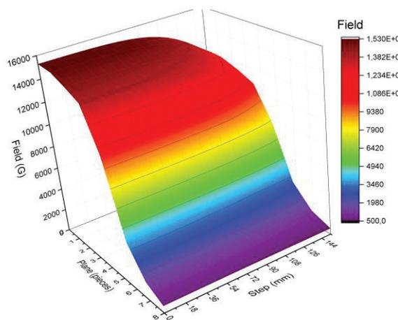
Figure 5: 3D map of the magnetic field for the SP-94 dipole magnet used in the new Nuclotron applied beamlines.
