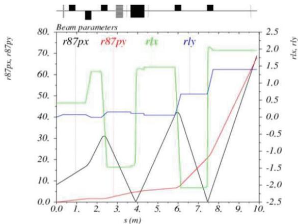
Figure 3: Dependences of horizontal and vertical beam sizes (95% of particles) on the beamline longitudinal coordinate.
