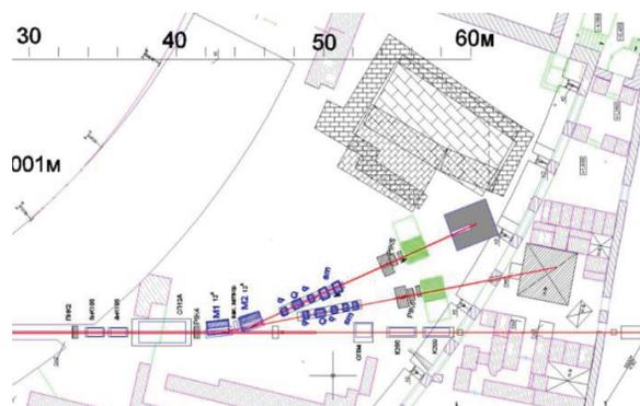
Figure 4: The new Nuclotron beamlines applied for radiobiological researches and chip irradiations.
