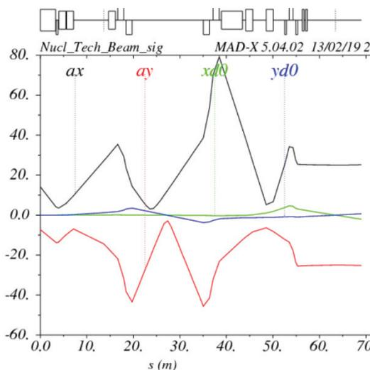
Figure 6: Dependence of the horizontal and vertical beam sizes (95% of particles) on the longitudinal coordinate of the Nuclotron beamline.
