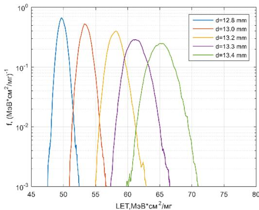
Figure 7: Spectrum of LET in the Si chip for <sup>197</sup>Au<sup>79+</sup> ions at the initial energy of 250 MeV/u after their deceleration in the polyethylene degraders of different thickness.
