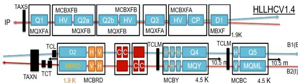
Figure 1: HLLHCv1.4 layout of the right side of IR1 and IR5 with quadrupoles (Q), non-linear corrector package (CP), dipoles (D), collimators and masks (TC), crab cavities (CC), and passive absorbers (TAX).
