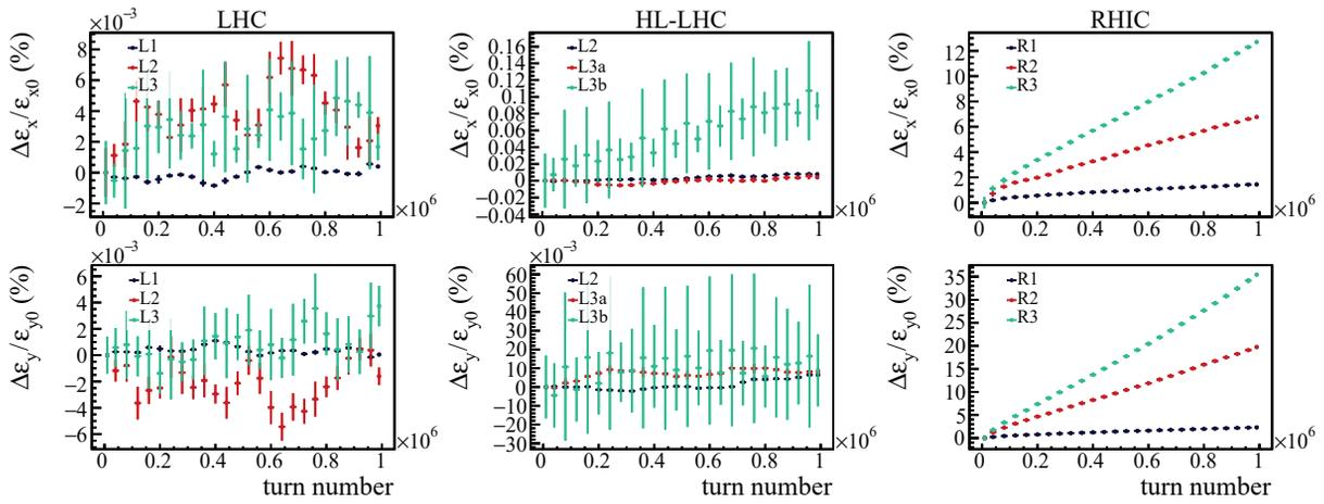
Figure 2: Relative horizontal (top) and vertical (bottom) emittance change vs. turn number for a Pb bunch in the LHC (left), HL-LHC (centre) and for a Au bunch in RHIC (right) for three different filling patterns.
