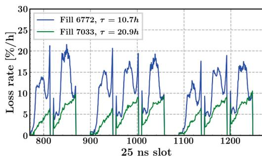
Figure 5: Bunch-by-bunch loss rate for three consecutive bunch trains at  $\beta^* = 33$  cm, for two fills performed before and after the lifetime optimization.
