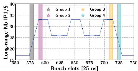
Figure 3: Number of BBLR interactions at each of the high-luminosity interaction points for the different bunches of a circulating bunch train. Groups of bunches that are analyzed in detail are highlighted in different colours.
