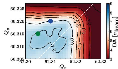
Figure 2: Simulation of DA as a function of the betatron tunes. Dots represent the chosen tune settings.
