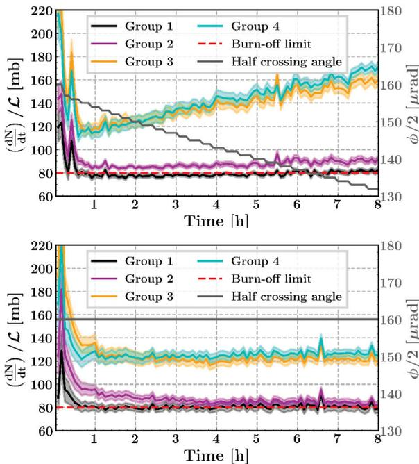
Figure 7: Effective cross sections during the time spent in collision for selected groups of bunches as illustrated in Fig. 3 during a typical fill with gradual crossing angle reduction (upper plot) and a test fill with constant crossing angle (lower plot).
