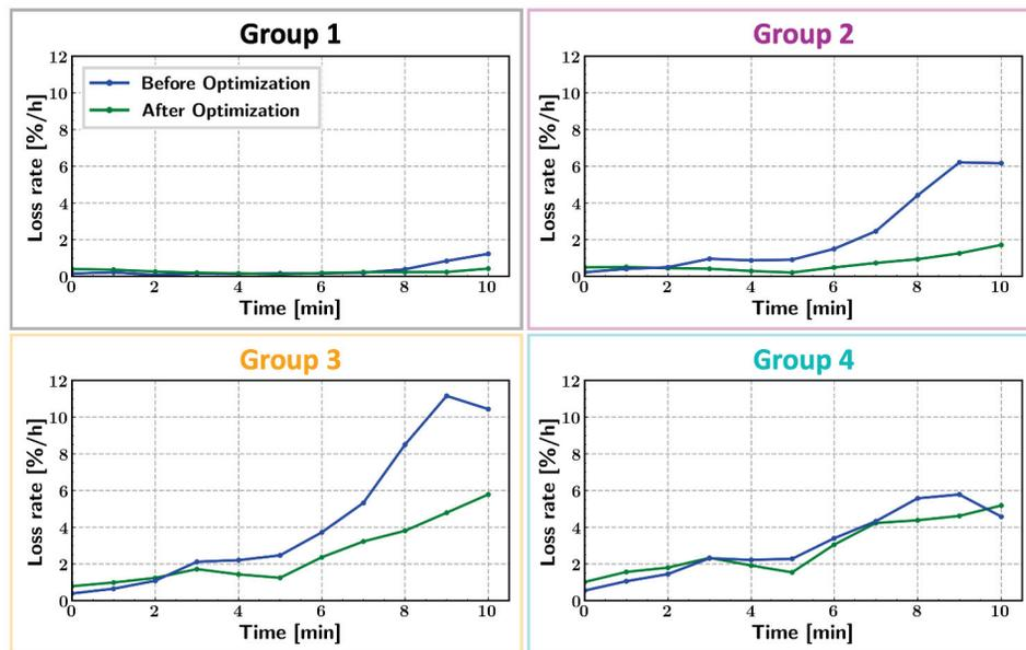
Figure 4: Loss rate measured for the groups of bunches illustrated in Fig. 3, before and after the optimization (average over several fills).
