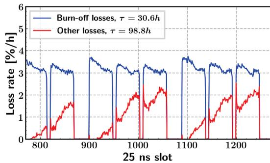
Figure 6: Bunch-by-bunch loss rate decomposition for three consecutive bunch trains 5.5 h after the start of collisions.
