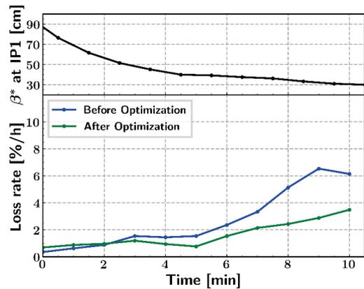
Figure 1: Top:  $\beta^*$  evolution during the betatron squeeze process. Bottom: beam loss rate during the betatron squeeze before and after the lifetime optimization.
