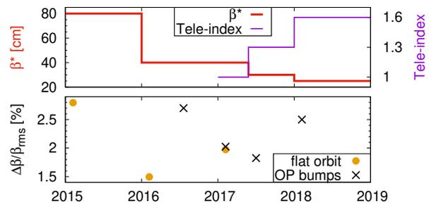
Figure 1: Run 2 at a glance:  $\beta^*$ , tele-index (top) and rms  $\beta$ -beating (bottom) averaged over the two planes and two beams, with and without operational (OP) crossing angle. Note that the 2016 measurement with OP bumps misses one plane out of four.
