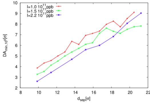
Figure 1: One-million turn DA as a function of the beam to beam normalized separation for the nominal intensity (blue) and lower values (green and red).
