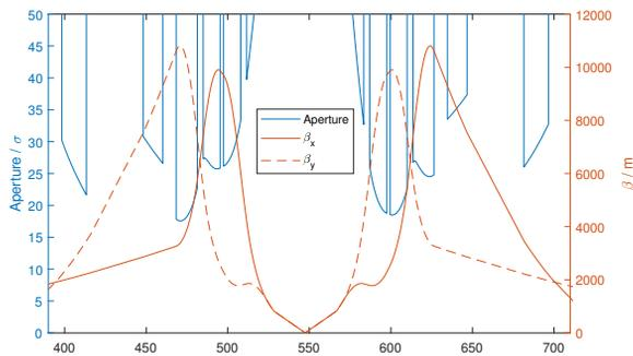
Figure 2:  $\beta$ -functions and BSC in HE-LHC triplet and separation dipoles for  $\beta^* = 0.45$  m.
