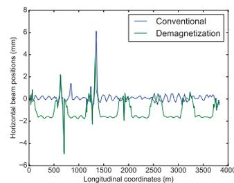
Figure 3: The horizontal orbit shifted inwards by 1.8 mm in the ring due to expected difference of RHIC dipole transfer function with the demagnetization cycle.
