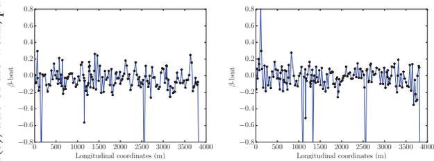
Figure 4: The measured relative errors of  $\beta$ -functions, the horizontal plane on the left and the vertical plane on the right, with the demagnetization cycle.
