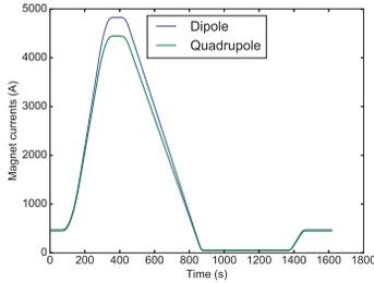
Figure 2: Conventional magnetic cycle: RHIC superconducting dipole and quadrupole currents are ramped up to currents for top energy, back down to park current at 50 A, then up to operating currents for beam injection.
