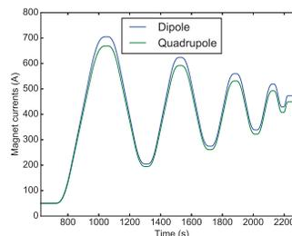
Figure 1: Demagnetization magnetic cycle: RHIC superconducting dipole and quadrupole currents are ramped up and down several times, with intermediate current points at [50, 700, 200, 625, 275, 560, 340, 520, 430 A], before being held constant at operating currents for beam injection.
