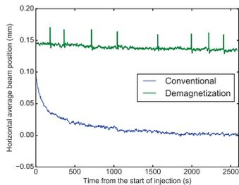
Figure 5: Comparison of the horizontal average beam position drifts, due to persistent currents decay in superconducting dipoles, with the conventional cycle (the blue curve) and the demagnetization cycle (the green curve).
