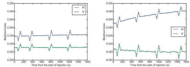
Figure 6: The left plot shows the drift of the horizontal and vertical betatron tunes after the demagnetization cycle. The right plot shows the drift of the horizontal and vertical betatron tunes after the conventional cycle. The excursion of the betatron tunes were due to change of RF frequency for chromaticity measurements.
