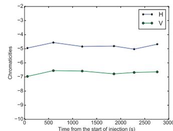
Figure 7: The measured beam chromaticities after the demagnetization cycle.
