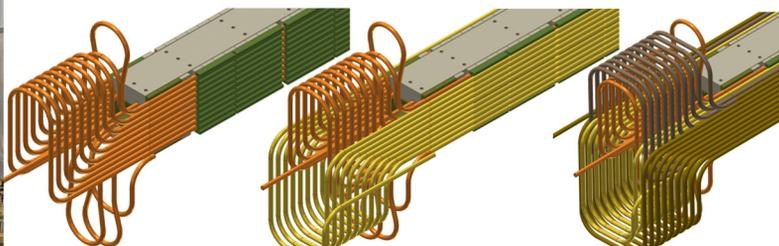
Figure 6: Winding the layers of a CIC block-geometry dipole: a) completed winding of 3 T JLEIC dipole; b) winding strategy for the 6 T CIC winding, showing the stages when successive layers are complete.
