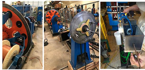
Figure 4: CIC manufacturing at ATC: a) 24-spool stranding machine; b) SS foil over-wrap; c) drawing of sheath tube onto cable.
