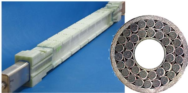
Figure 3: a) FRP support beam, formed by assembling 'window-frame' segments of G-11 FRP onto the 316SS beam tube, vacuum-impregnating the assembly, and precision-machining the half-round channels that position each CIC turn; b) cross-section photo of 2-layer NbTi CIC.
