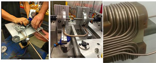
Figure 2: Robotic bending tools used to form a) the 180° bend and b) the 90° saddle bend that comprise the end geometry of each winding turn; c) a completed 24-turn end region of a 3 T CIC dipole.
