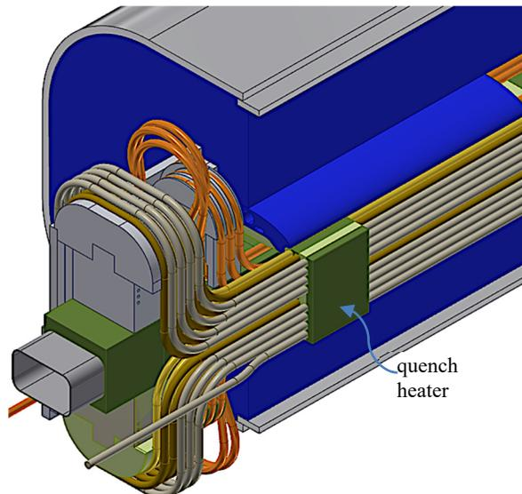
Figure 1: Cutaway of the 6 T CIC dipole design, showing the FRP structure, the 4-layer CIC winding, the beam tube, the steel flux return, and a quench heater.
