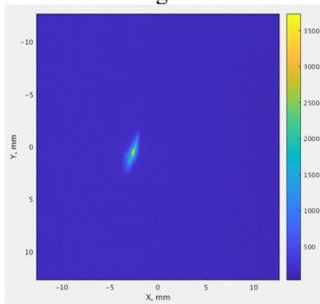
Figure 2: Image of the compressed and accelerated beam in the dogleg profile monitor. The dispersion is 1.2 meters and beam energy spread is  $3 \times 10^{-3}$ .
