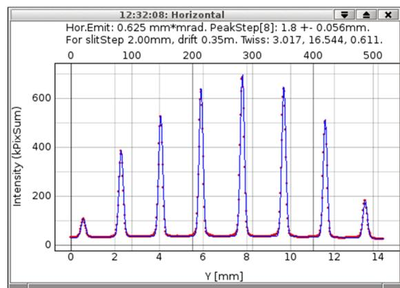
Figure 3: Emittance measurement of 0.75 nC bunch with slits.
