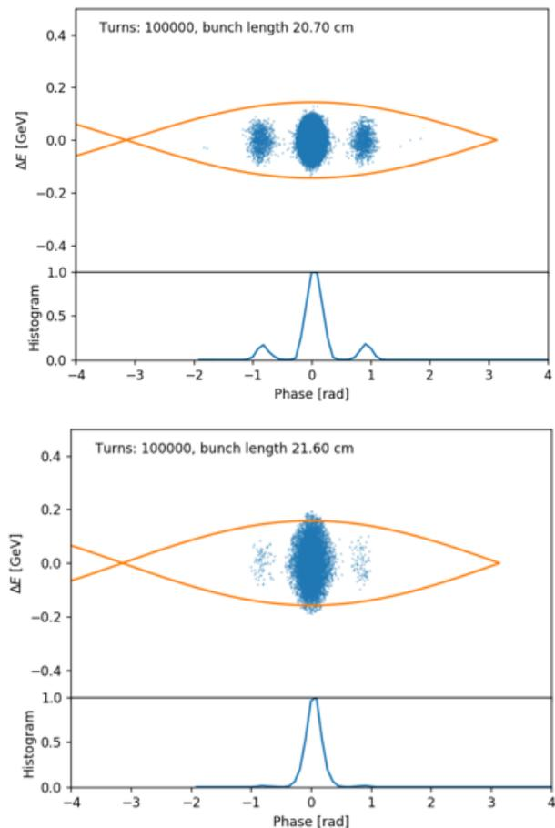
Figure 3: Particle distribution in 28 MHz torus with 56 MHz cavity turned off (left) and at 2 MV (right). The orange line outlines the 28 MHz cavity bucket.
