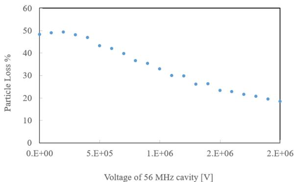
Figure 4: Particle loss with 56 MHz at different voltage.
