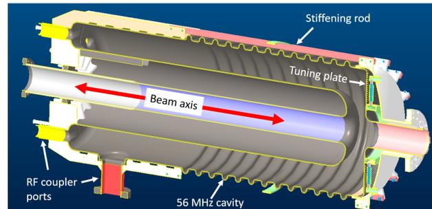
Figure 1: Crosssection view of the 56 MHz SRF cavity.
