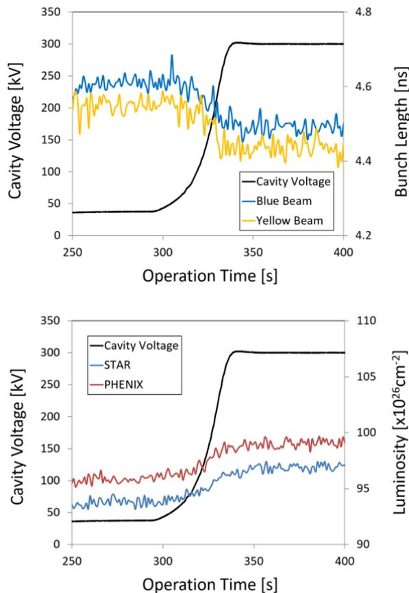
Figure 2: Bunch length decrease (left) and luminosity increase (right) directly related to 56 MHz cavity in operation.
