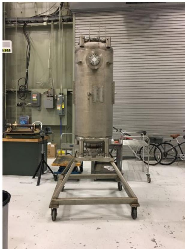
Figure 5: 56 MHz cavity with helium vessel after disassembled from cryomodule.
