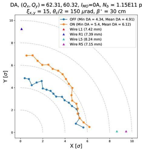
Figure 1: DA with (orange) and without (blue) BBCWs. The wires transverse positions are indicated by the triangle markers.
