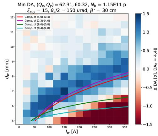
Figure 2: Minimum DA as a function of the beam-wire distance  $d_w$  and the wire current  $I_w$ . The longitudinal position of the wires is the one in the present LHC. The scale is given with respect to the DA of the machine without wires ( $4.48 \sigma$ ). The colored lines represent the function  $I_w(d_w)$  needed to compensate a given RDT.
