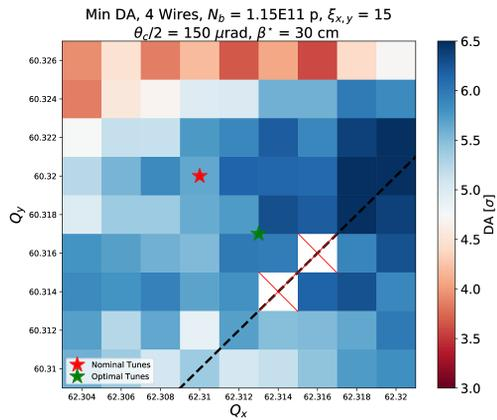
Figure 4: Minimum DA as a function of the vertical and horizontal tunes, with wires ON. The red crosses show the missing points in the study (no DA value).
