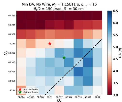
Figure 3: Minimum DA as a function of the vertical and horizontal tunes, without wires.
