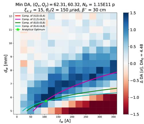
Figure 5: Minimum DA as a function of the beam-wire distance and the current carried by the wires in the LHC. The scale is given with respect to the DA of the machine without wires ( $4.44 \sigma$ ).
