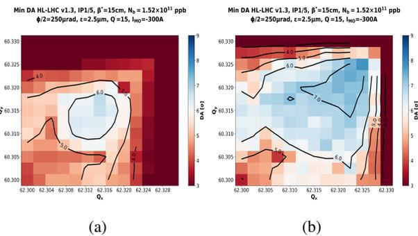
Figure 4: The minimum DA for different working points: (a) the ultimate scenario of HL-LHC and (b) the ultimate scenario of HL-LHC with wire compensators.
