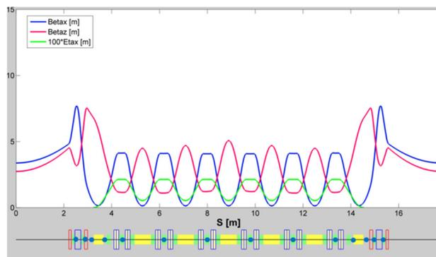
Figure 2: 20 × (7BA HOA lattice) studied in this contribution. Yellow - bends; Vertical rectangles - quads (red QD, blue QF); green - sextupoles; blue circles – octupoles.
