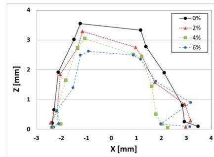
Figure 6: Dynamic aperture with 6D tracking with respective 6 families of sextupoles and octupoles.
