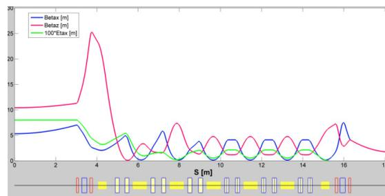
Figure 7: Symmetry 4 7BA HOA lattice with 8 cm of horizontal dispersion in the long straight to accommodate longitudinal injection [10].
