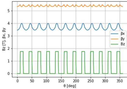
Figure 3: Beta functions and  $B_z$  of PPR.
