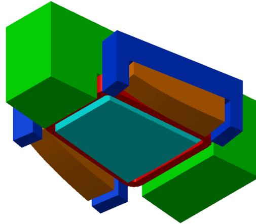
Figure 5: 3D model of the electromagnet of PPR.
