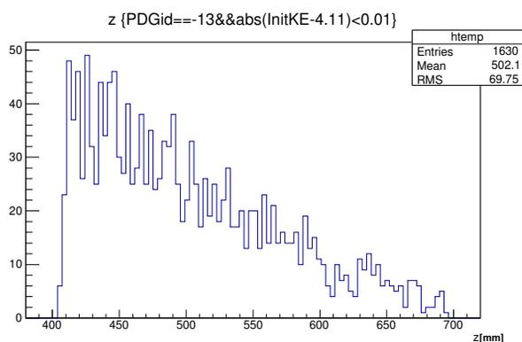
Figure 2: Initial distribution of the surface muons on the production target. Center of the target is at  $z = 550$ .
