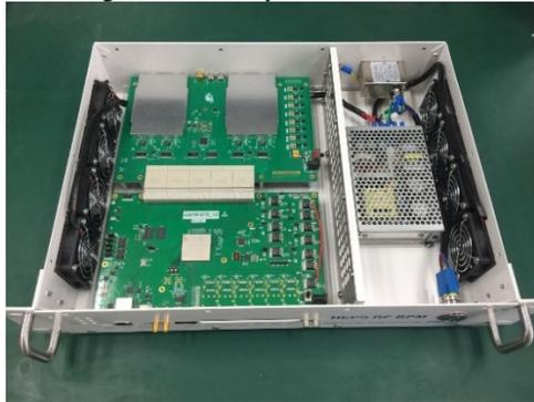
Figure 6: The beam position monitor electronics.
