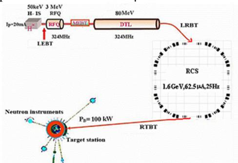
Figure 1: Layout of China Spallation of neutron Source.
