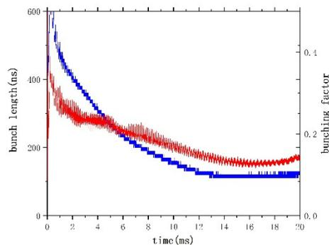
Figure 7: Bunch length (blue) and bunching factor (red).
