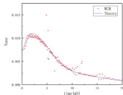
Figure 8: Tune measured from WCM and theoretical calculation.
